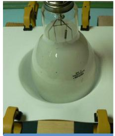
Plunge-moulding the internal fuel tanks.
