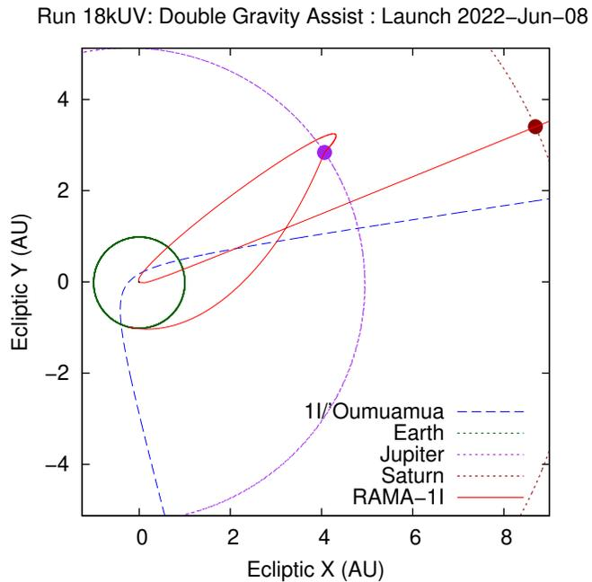
This is a good early launch trajectory, using Jupiter, the Sun and Saturn to speed Lyra on its way. With a launch in March 2022, the 1I flyby is in early 2043 at a distance of about 146 AU, with a payload about the size of *New Horizons*,  $\sim 500$  kg possible with a SLS sized launch vehicle. Unfortunately, the double gravity assists are not possible one synodic period (13 months) later, due to the relative motions of Jupiter and Saturn, and won't repeat for 30 years.
