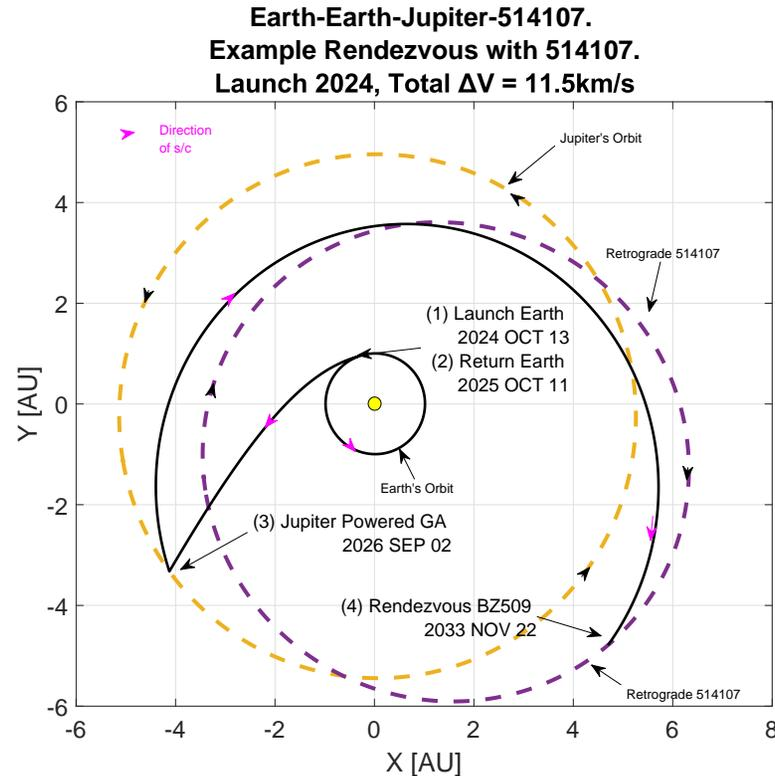
This is a mission to a Type 6 object, a **possibly** captured ISO in a retrograde orbit. Retrograde orbits have large velocities relative to our prograde orbiting spacecraft, but Adam Hibberd found a Jupiter gravity assist that would make a BZ509 orbiter or lander possible with reasonable total velocity.
