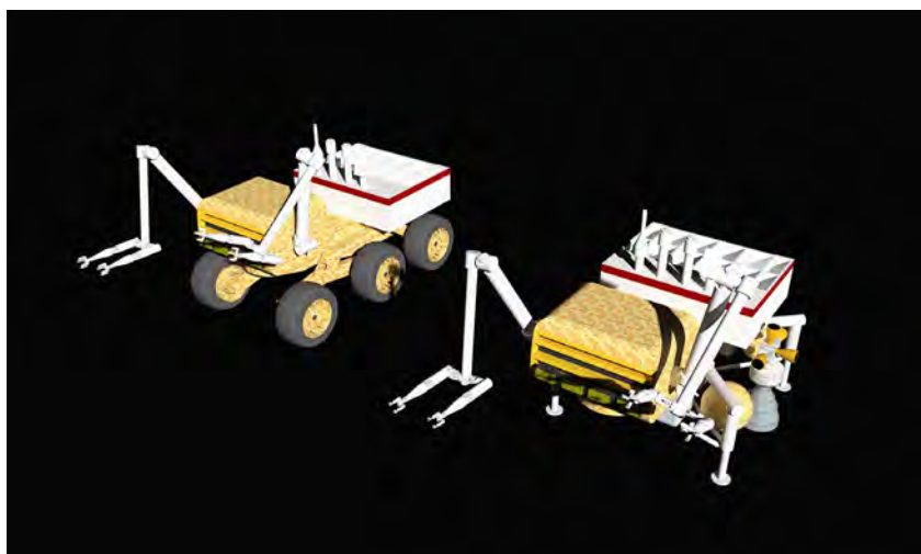
Image 5- Geologist, ground and space versions. Commonality reduces the number of parts required for production. A modern reference would be the NASA MMSEV.
