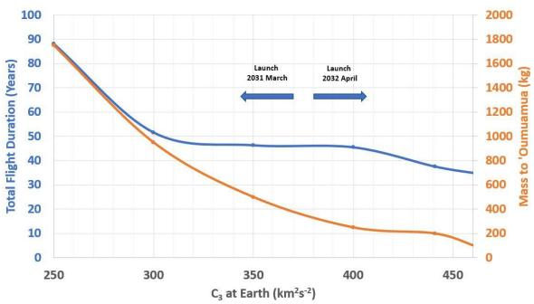
In this Figure the horizontal axis,  $C_3$ , is a measure of the energy per unit mass of the escape orbit from Earth. For any given launcher (in our case the SLS Block 2B + Centaur + STAR 48BV), the lower this  $C_3$  value then the higher the payload mass delivered to the escape orbit in question.
