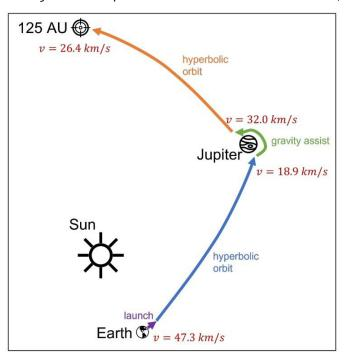
Illustration of the dark matter explorer spacecraft's proposed trajectory from Earth to 125 AU (not to scale). Included speeds denote spacecraft's speed relative to the Sun at points of interest.
