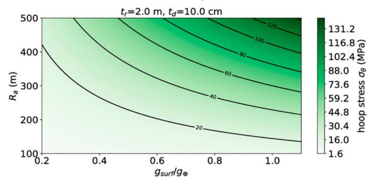
Hoop stress for an asteroid spun up to form a cylindrical shell of thickness 2 m and contained in a scaffold of thickness 10 cm. The asteroid is assumed to have a uniform density of 1 g/cm<sup>3</sup>. The vertical axis is the radius Ra of the asteroid, in meters. The horizontal axis is the surface gravity of the asteroid in units of Earth surface gravity.
