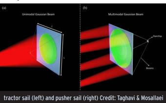
Their paper discusses in detail - nanoscale photonic unitcell design and an optomechanical analysis framework. It advocates a dual-pattern metasail with uni-modal beam with the nanocraft placed at the back-side of a sail (pusher configuration) using an all-dielectric metasurface.
