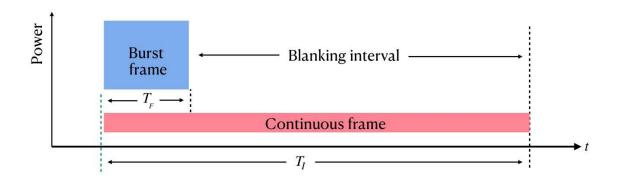
An illustration of burst-mode transmission, in which a section of transmitted signal of duration T<sub>1</sub> is compressed into a shorter duration T<sub>2</sub> < T<sub>1</sub> at higher power, so that the total energy is not affected. This creates a blanking interval known to the receiver, during which there can be no signal photon detections and any background photons can be ignored.
